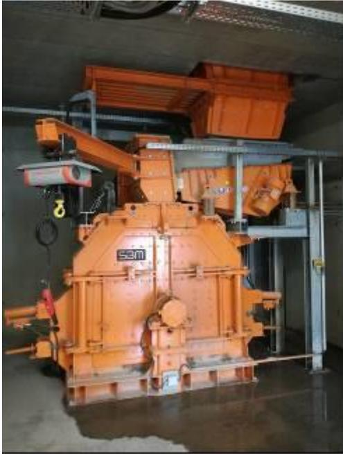
*Bild 3: The SMR 10/5/4 Impact Crusher made by SBM crushes the oversize fractions to re-integrate them into the production cycle.*
